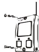
5. Mount the Wall Console to the wall with 2 screws.
