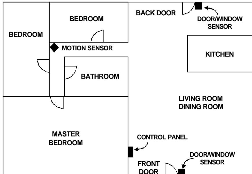
You may choose to install a motion sensor to protect any valuables such as antiques or paintings. Point the motion sensor directly at the valuables and if they are disturbed in any way the alarm will be sounded.
