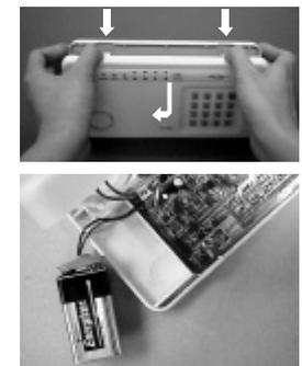
Note: To guard against sabotage, the Control Panel is equipped with an emergency switch that activates the alarm instantly when the case is opened. Make sure that the unit is disarmed when you open the case or you will activate the alarm.
