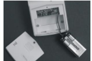
Insert 9V alkaline battery to the sensor
