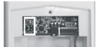
Sensitivity Connectors on Motion Sensor
