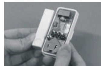
When the magnetic contact is closed, the receiver will not beep.
