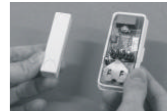
When the magnetic contact is broken (open), the receiver will beep and a LED will flash.
