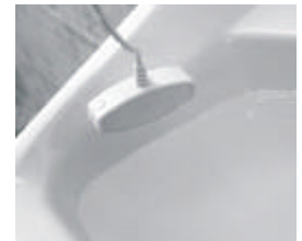
Remove the sensor portion from the water, receiver stops beeping and red LED stops flashing.
