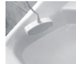
Remove the sensor portion from the water, receiver stops beeping and red LED stops flashing.
