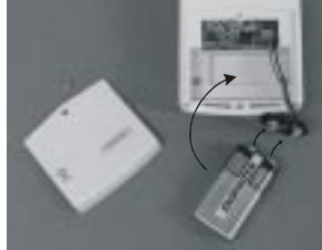
Insert 9V alkaline battery to the sensor
