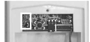
Sensitivity Connectors on Motion Sensor
